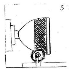
Presenting the tool at an angle will create small diagonal grooves. The method of changing the pattern of diagonal grooves can be achieved by presenting the tool at different angles.
